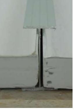
View of top of Rear Baffles. Remove spacers and screws, and use to install upper Baffles.
